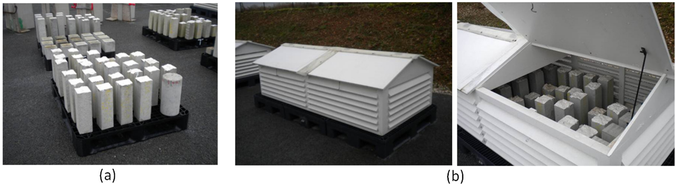
Fig. 7. Concretes exposed to (a) unsheltered and (b) sheltered conditions at Lyon.
